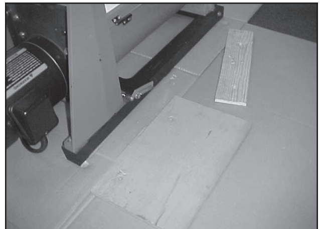
Fig. 3 Remove packing plates
