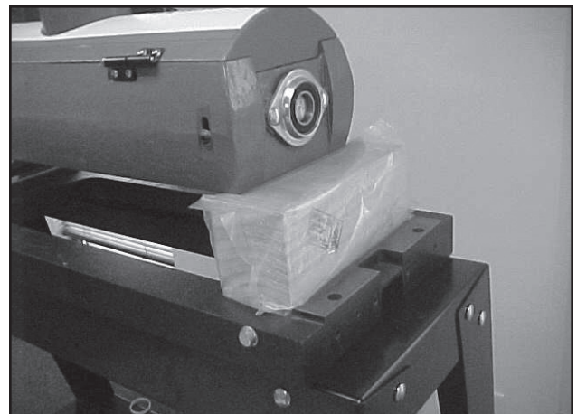
Fig. 4 Secure to stand, remove packing block
