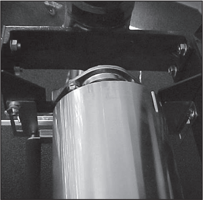
Fig. 11A Tension roller and depth gauge adjustment.
