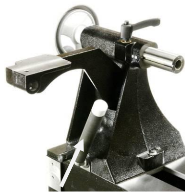
Tailstock clamp handle
